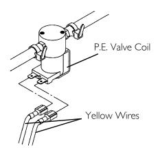
FIGURE 24.4 P.E. Valve Coil Test
