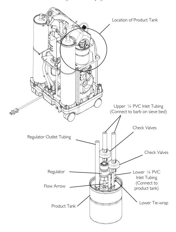
FIGURE 10.1 Replacing Check Valves
