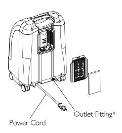
\*NOTE: This outlet fitting is to be used only for filling oxygen cylinders with the HomeFill home oxygen compressor. The outlet fitting does not affect concentrator performance. Refer to the HomeFill owner's manual, part number 1100873, for connection and operating instructions. When not in use, the plug provided with the concentrator should be inserted into the outlet fitting. For more information about the HomeFill, contact your Invacare dealer.
