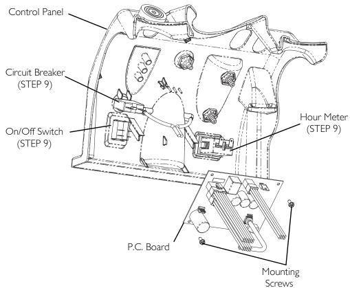
FIGURE 13.1 Removing Control Panel
