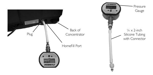
FIGURE 25.2 Pressure Testing
