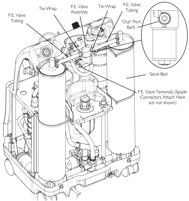
FIGURE 8.1 Replacing P.E. Valve
