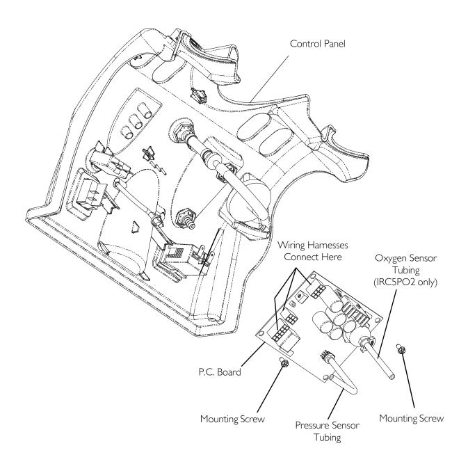
FIGURE 15.1 Replacing P.C. Board
