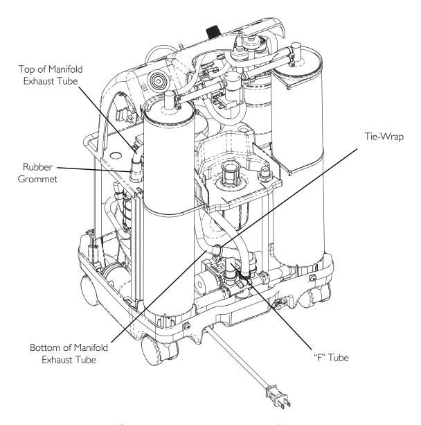
FIGURE 6.4 Replacing the Muffler Assembly
