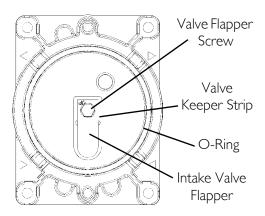
FIGURE 7.5 Removing Compressor and Compressor Heads - Rebuilding the Compressor - O-ring, Intake Valve Keeper and Valve Keeper Strip
