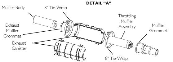
FIGURE 6.5 Replacing the Muffler Assembly
