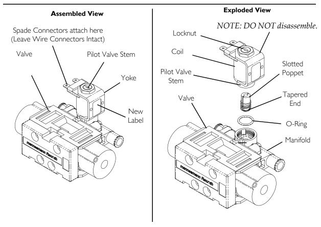
FIGURE 20.2 Replacing Pilot Valve Poppets and O-Rings
