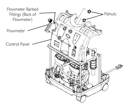
FIGURE 18.1 Replacing Flowmeter
