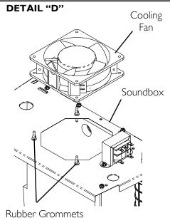
NOTE: Cooling fan removed from rubber grommets to show proper installation of grommets in soundbox.
