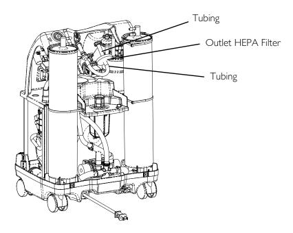
FIGURE 6.2 Replace the Outlet HEPA Filter
