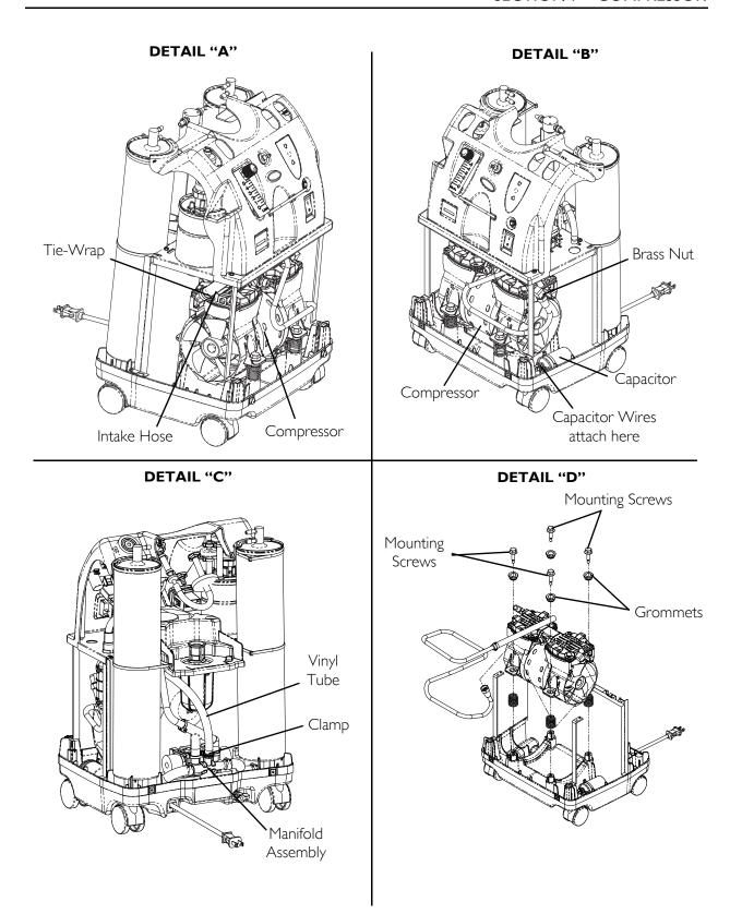
FIGURE 7.1 Replacing Compressor Assembly
