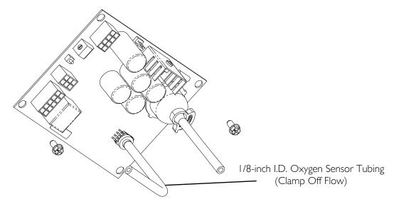
FIGURE 24.3 Oxygen Sensor
