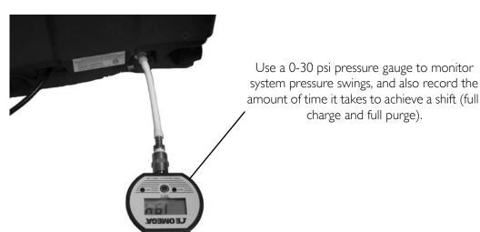
FIGURE 23.2 4 Way Valve Function Test
