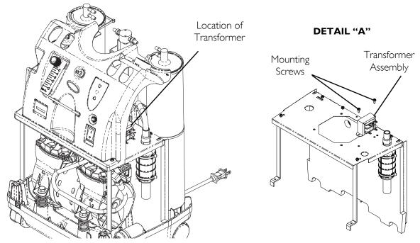
FIGURE 16.1 Replacing the Transformer
