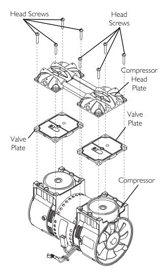
FIGURE 7.3 Removing Compressor and Compressor Heads - Rebuilding the Compressor - Compressor - Compressor Head Plate - Valve Plates
