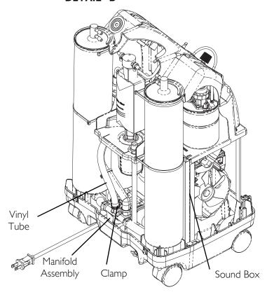
FIGURE 12.1 Replacing Heat Exchanger Assembly
