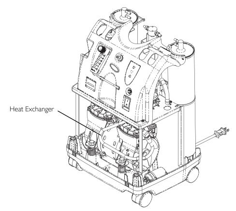
FIGURE 6.6 Cleaning the Heat Exchanger
