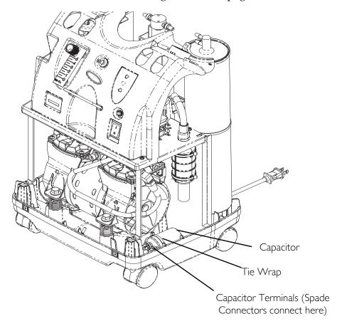
FIGURE 7.2 Replacing Capacitor
