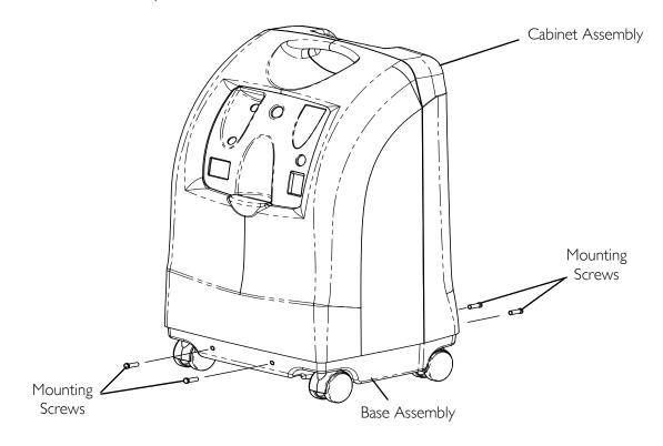
FIGURE 5.1 Removing Cabinet
