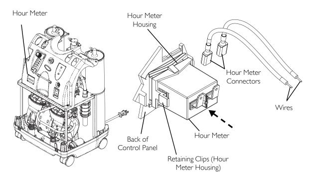
FIGURE 19.1 Replacing Hour Meter
