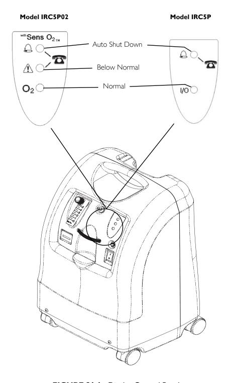
FIGURE 21.1 Display Control Panel
