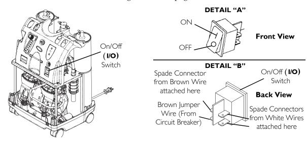
FIGURE 17.1 Replacing On/Off Switch
