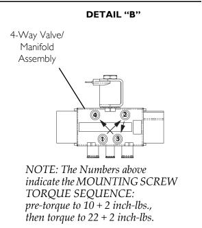
FIGURE 20.1 Replacing 4-Way Valve and/or Manifold Assembly
